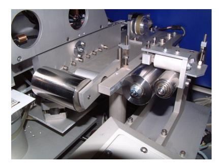
WAFER BREAKER BRK-60R is easy to use for singulating very small components, up to 2.5x2.5" wafer or substrate Robust; the Breaker unit is immediately operational, with minimum training. Vertical targeting is carried out with a video camera, for angular alignment. Monitor display includes an electronic crosshair. All parameters are directly adjusted on operator control panel.
